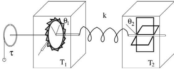
Fig. 2. Ratchet, pawl and spring Brownian motor.
