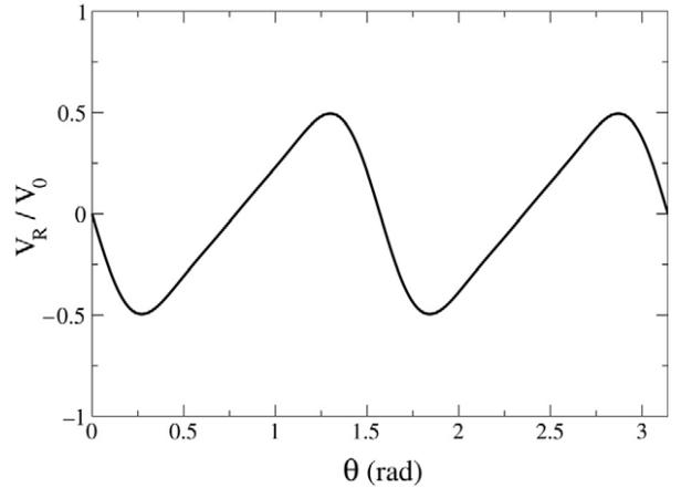
Fig. 3. Shape of the ratchet potential  $V_R$  for  $d = 4$ .
